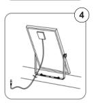
Fix the solar panel with wing screw.
